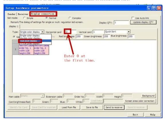
And then you will see the following window. Enter 3 in the blank for Horizontal card; enter 2 in the blank for Vertical card.
