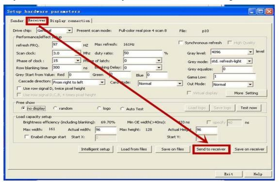
Step 12 Go back to the Display connection and click Send to receiver the third time.
